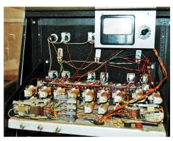
General Electric engineers here. Yola works in the Cathode Ray Tube Department, Bldg. 6. The tic-tac-toe machine was created by GE engineers Bert Liner, Bob Thor and Bob Hill." The machine was truly a marvel of design – since its' logic basically consisted of a number of hardwired latching and stepping relays. By the way, Jeff Houck-N2LYR now has this unit and is trying to get it functioning again.
